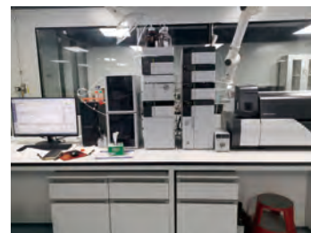
细胞微流控芯片-液相-质谱联用分析仪 Cell Microfluidic Chip-ultra High Performance Liquid Chromatography-triple Quadrupole Mass Spectrometer
